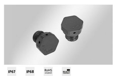
The new pressure compensation element PCE with M12  $\times$  1,5 thread is used to avoid variations in pressure caused by differences in temperature and thus, to prevent damage caused by condensation. It provides protection class IP68.
