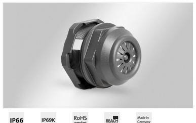
In enclosures and housings with a high degree of protection, temperature differences result in condensation. By using a drainage device, it is possible to safely drain off the condensate without losing a maximum enclosure protection of IP66. A water-permeable membrane ensures the drainage of the enclosure due to its capillary effect. The design prevents splash water from entering the interior of the enclosure.
